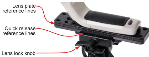
Attach lens with lens plate by loosening lens lock knob completely, then place lens plate into quick release. Tighten lens lock knob completely, then loosen 1/2 turn. Slide lens forward or backward to balance, then retighten lens lock knob.
