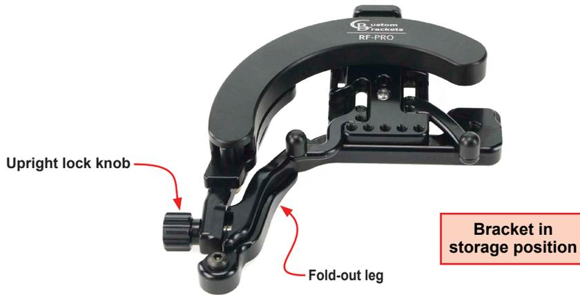
Remove your camera and flash prior to storage. It is not necessary to remove a flash cord if attached to the flash mounting plate. Loosen the upright lock knob and rotate upright backward to lower until flat. Fold in the leg.
